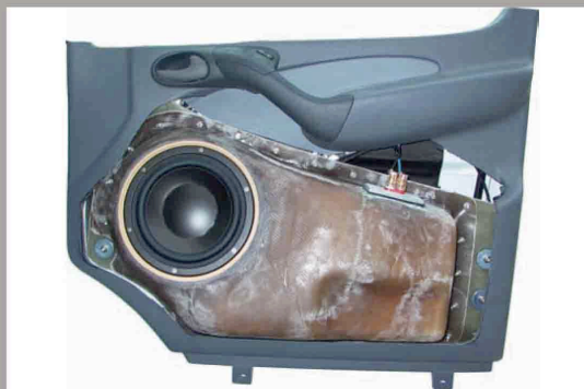
View of partially completed door enclosures.
