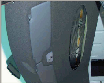
View of the completed headliner.
